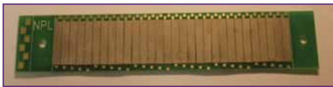
Figure 1. Macro sized piezoelectric energy harvesting cantilever
